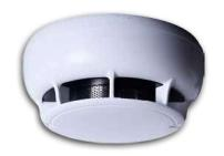
TFD-3230 Conventional Optical Smoke Detector uses genuine smoke chamber perfected by Teknim engineers through long term fluid mechanics and optic refraction tests. Fire is detected by optical sensing technology. Detector has a series of algorithms developed to minimize erroneous detections and to provide pollution warning. Smoke chamber can be easily removed for cleaning in case of possible pollutions in excessively dusty environments.
